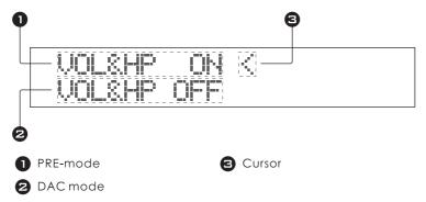
Turn the volume/channel control knob to switch the cursor to the working mode you need, then press it, so that MINI-i will save the settings automatically, and work under that mode.
