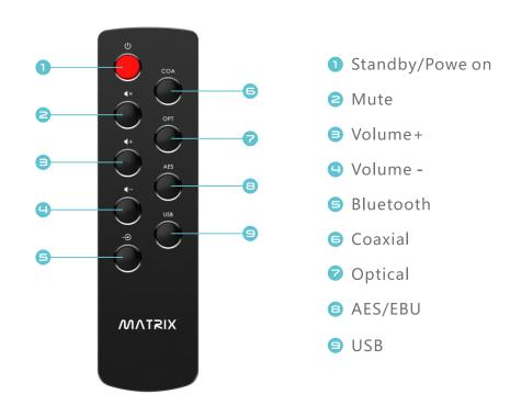
Long press any button for 2 seconds into the auto scan mode.
